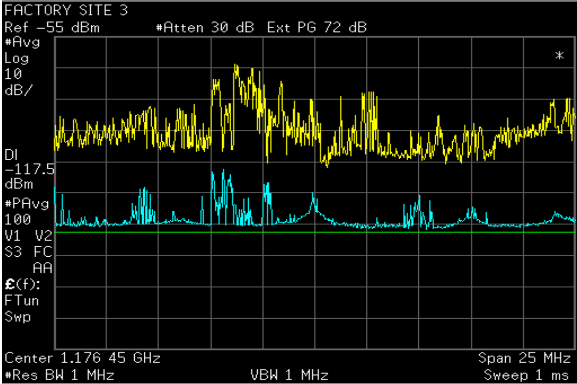
Figure D-114. Ambient Emissions in GPS L5 Frequency Band at Factory Site #3.
