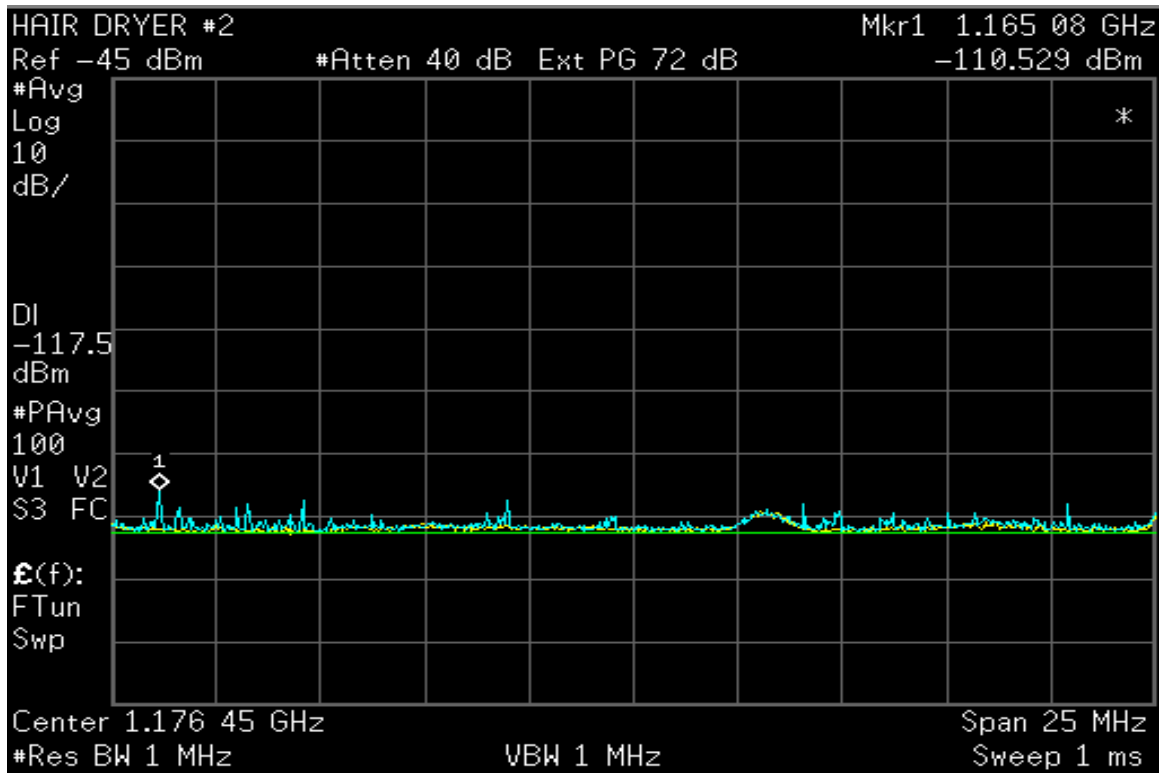
Figure E-155. Electric Hairdryer #2 Radiated Emissions in the GPS L5 Frequency Band.
