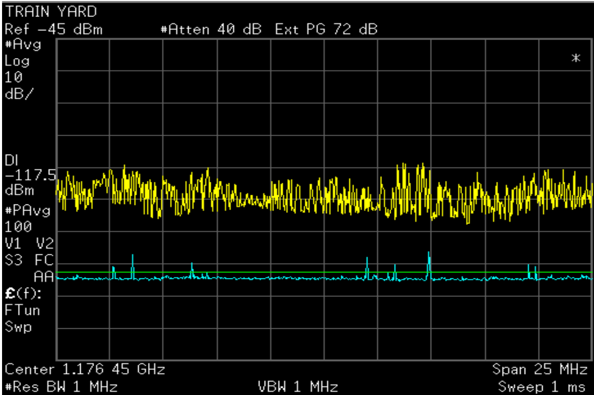
Figure C-52. Ambient Emissions in the GPS L5 Frequency Band at the AMTRAK Train Yard.
