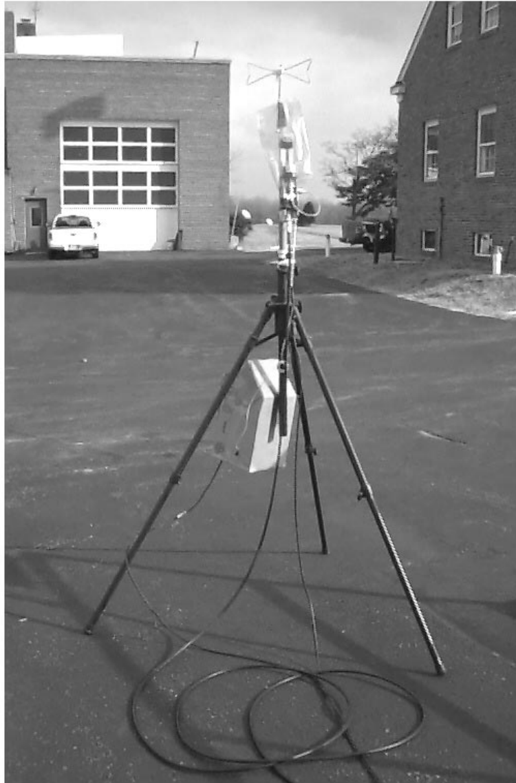
Photo F-6. Tripod-Mounted Bowtie Antenna with Preamplifier and Remote Spectrum Display Viewing Box
