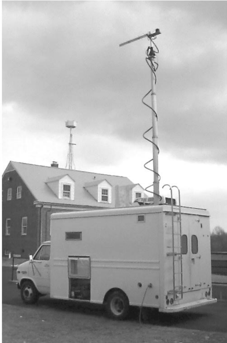
Photo F-2. Port Side View of Vehicle with Antenna Mast Extended
