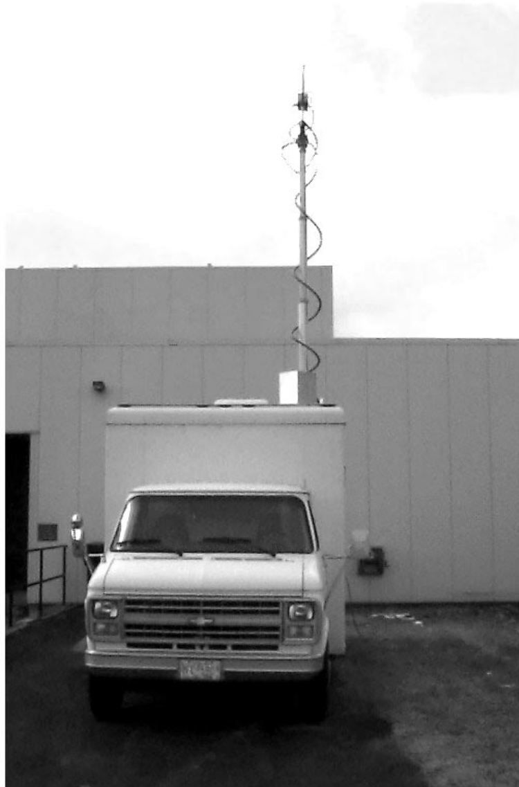
Photo F-1. Front View of Vehicle with Antenna Mast Extended
