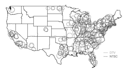
Channels 52 to 59: DTV & NTSC Incumbents Adjacent and Co-Channel Protection Zone
